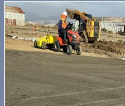
Drive-over radiological scans of material on RSY pads
