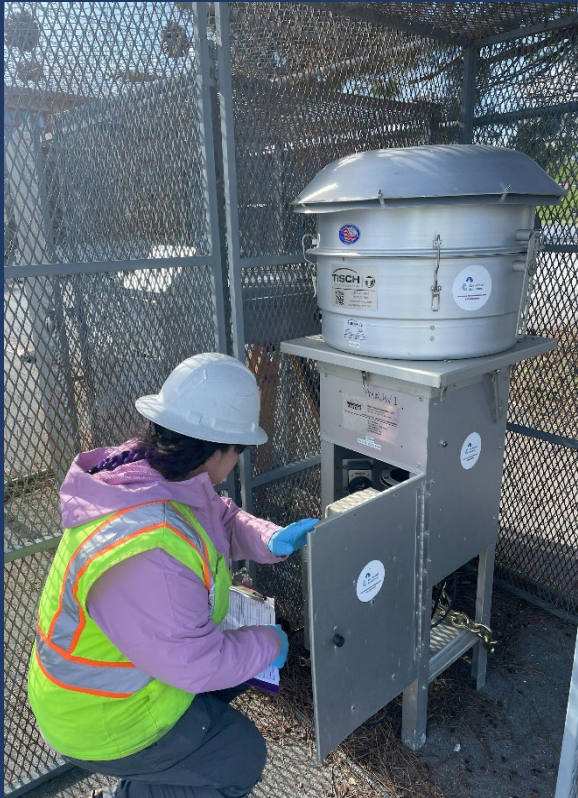
Gathering readings from high volume air monitor
