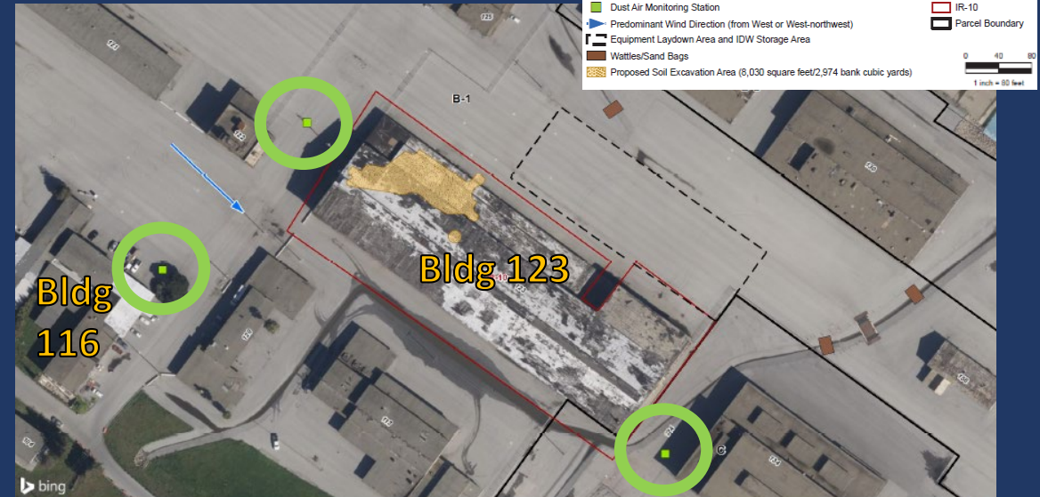
Location of air monitoring stations during Building 123 demolition, approximately 10 feet from each respective building
